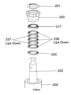
10. Reassemble intake valve (213) as shown.
